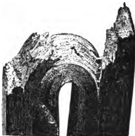
FIG. 54.—FRACTURE AT ORDINARY TEMPERATURE.
